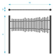
The Sonora's 21 tubular bells produce a tone that is bright, clear, and resonant. Made from hand-tuned, heavy duty anodized aluminum, the Sonora can be wall-mounted or affixed to posts for easy installation in any location.
