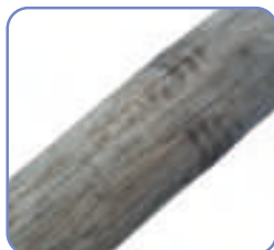
Non-impregnated robinia wood with a natural weathered patina
